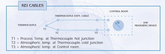
Range of Thermocouple Extension/ Compensation cables :-
