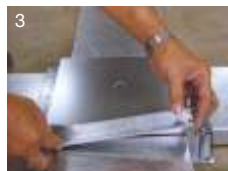
3 Align the trap frame bracket with the side blank plate
