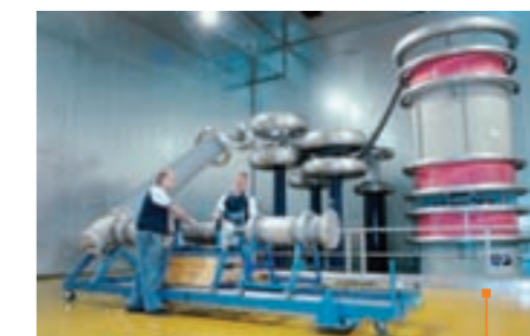
Final testing: Every joint is tested individually to ensure 100 % performance.
