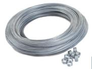
under strict guidance of technical personnel. The diameter ranges from 0.19 mm to 1.20 mm in bright finish and 0.50 mm to 6.0mm in matt finish (coated) in grade of AISI 302, 304 & 316, 321, Standard ASTM A313 and others.
